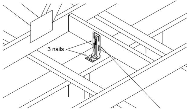
**Trusses at right angle to bracing wall**
