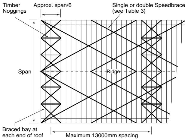
b) For jack trusses or rafters, use single Speedbrace in an 'X' configuration and the angle of Speedbrace to end wall should be between 30° and 45°.
