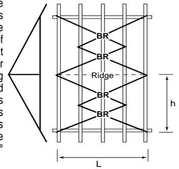
2. **Short Roofs.** Where the roof length "L" is of length to give a brace angle between 30° and 45° then only one bay of bracing is required each side of the ridge line as shown.
