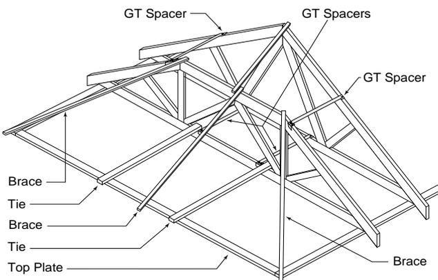
Each successive truss should be spaced using GT Spacers. GT Spacers are recommended in lieu of gauging rod or timber ties, as these can be fixed to the trusses prior to lifting trusses on to top plates.
