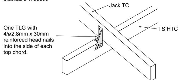
**Detail E2 - Jack Truss to Hip Truss (maximum jack station 2400mm)**
