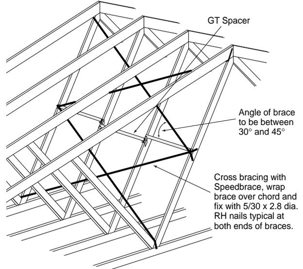
The GT Spacer can also be used as permanent lateral bracing for webs in standard roof trusses for domestic constructions. The GT Spacer can be used as a web tie where truss designs require bracing to be applied to webs for the following conditions.
