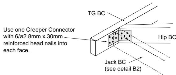
**Detail B2 - Jack Truss to Truncated Girder Truss**
