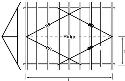
3. **Long Roof** – where the roof length "L" is 3½ to 4 times the half span "h" of the roof truss.
