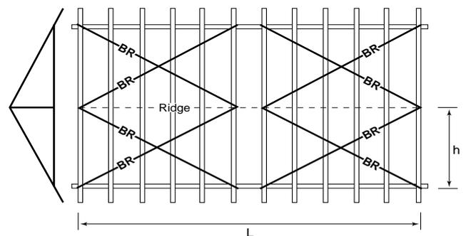
For a roof with overall truss span greater than the maximum values specified in Table 2, but less than 13.0 m, use a double Speedbrace as shown below.
