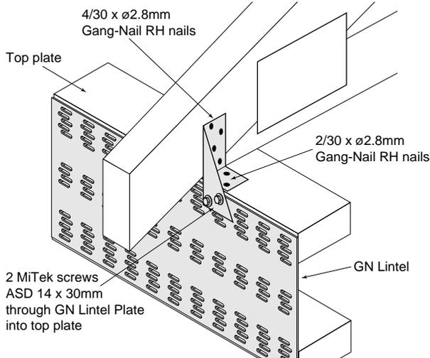
In cases where Trip-L-Grips will need to be fixed through the GN Lintel Plate, two MiTek screws ASD 14 x 30mm long may be used in place of 4 x 2.8 diameter nails into side of top plate to assist with the penetration of the GN Lintel Plate.
