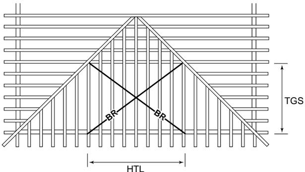
3. Where the horizontal top chord length (HTL) is longer than 1.5 times the truncated girder station (TGS).
