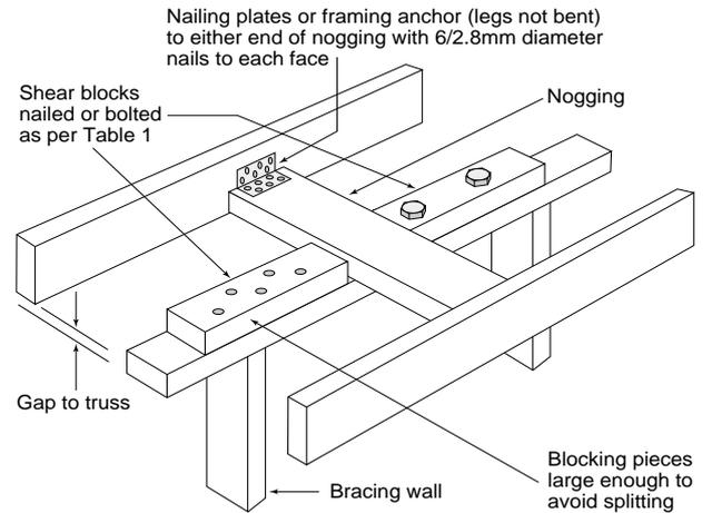
**(c) Non-Load Bearing External Wall**
