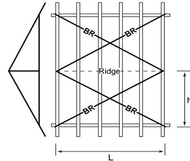
3. **Long Roofs.** Where the roof length "L" is long compared to the half span "h" of the roof trusses and would result in a brace angle less than 30°, two or more crossed bracing bays are required each side of the ridge to ensure the brace angle is between 30° and 45° as shown.
