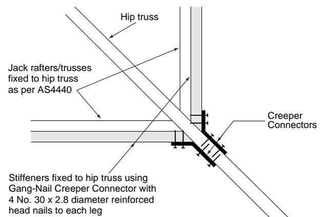
Detail C. Fixing of Hip Truss to Truncated Girder Truss
