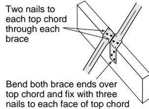
5. At the heel, Speedbrace should be fixed in one of the following ways:-
