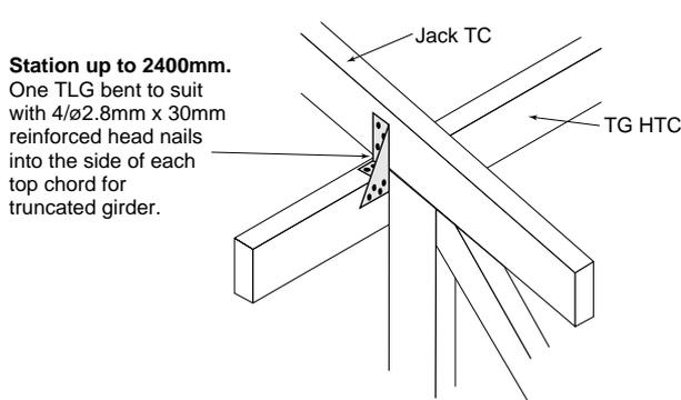
**Detail B2 - Jack Truss to Truncated Girder Truss cont.**
