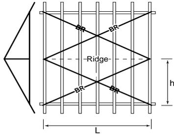
2. **Short Roof** – where the roof length "L" is 1½ to 3½ times the half span "h" of the roof truss.
