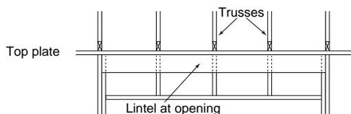
Top plate strengthening may be required where trusses do not coincide with studs.
