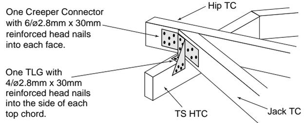
**Detail D2 - Extended Jack or Hip Truss to top chord of Truncated Standard Trusses**
