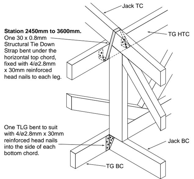
**Detail C2 - Intersection of Jack and Hip Truss to Truncated Standard Truss**
