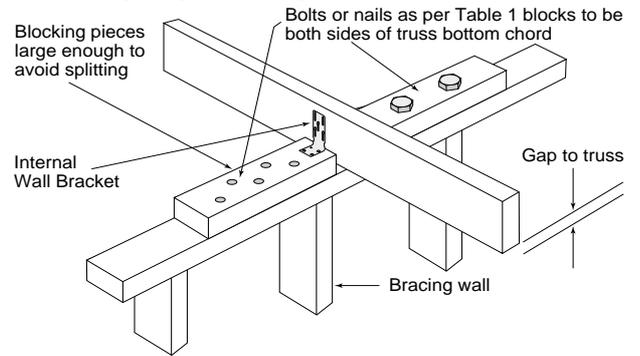
**Trusses parallel to bracing wall**
