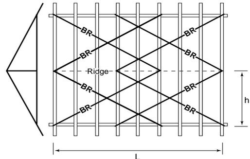
4. **Very Long Roofs.** As for long roofs, except continue bracing for length of building such that each truss is crossed with at least four braces.
