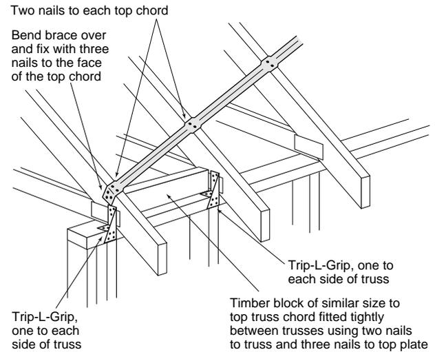
Where the standard trusses are supported by a girder truss or a beam rather than a wall top plate, fix Speedbrace at truss heel as shown following.
